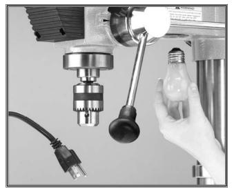
Figure 17b. Installing a light bulb.
